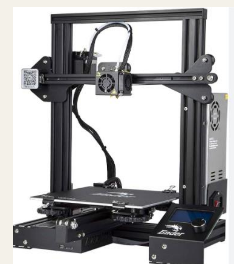
Figure 7: 3D Printer with Extruder under testing
