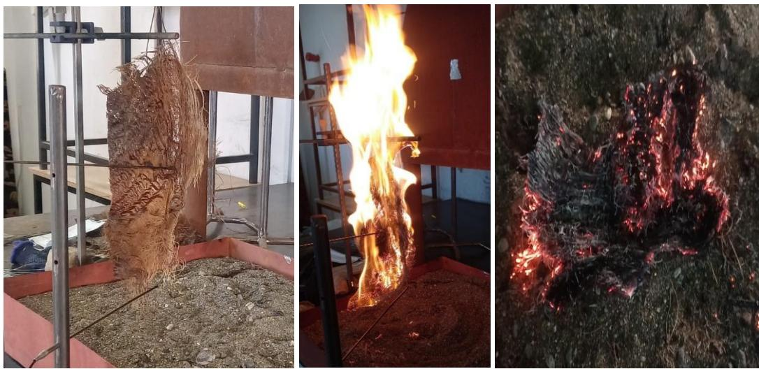
Figure 18. Leaf sheath in vertical with fire.
