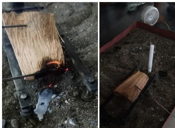
Figure 26. Trunk in horizontal with fire.
