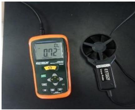
Figure 7. Anemometer device.
